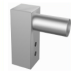
L shape pole mount adaptor Q235+SPCC materials with hot dip galvanizing, for 100x100mm square pole. Code: SP-R03-10
