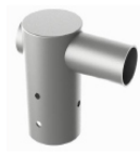
L shape pole mount adaptor Q235 materials with hot dip galvanizing, for dia.90mm pole Code: SP-R03-09(for dia.90mm) Code: SP-R03-09 a(for dia.76mm) Code: SP-R19-01(for dia.60mm)
