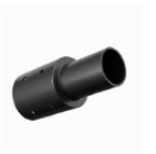
Post top mount adaptor Q235 materials with hot dip galvanizing, 76mm to 60mm Adaptor Code: SP-R03-16 (for dia 76mm pole)
